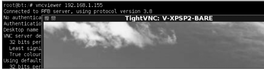
Figure 4-18: Connecting to VNC with no authentication using vncviewer
