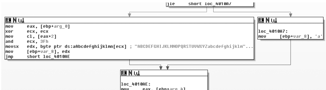
Figure 14-2L: Base64 encoding function (0x401000) with alternative padding
