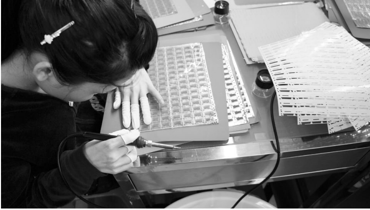
A worker manually aligning coverlay onto flex-circuit material
