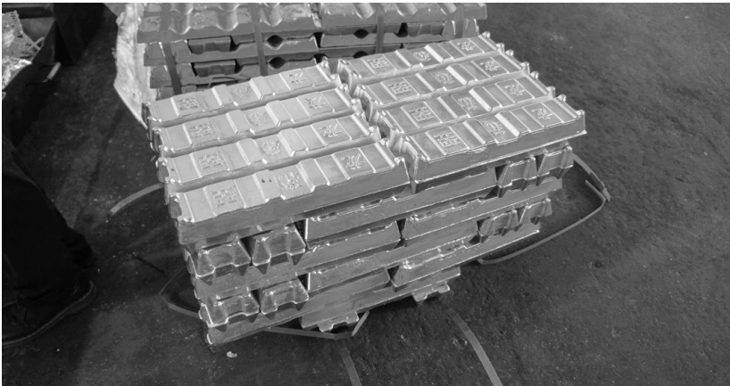
Approximately 1 ton of ingots, composed of 93 percent zinc and 7 percent aluminum alloy
