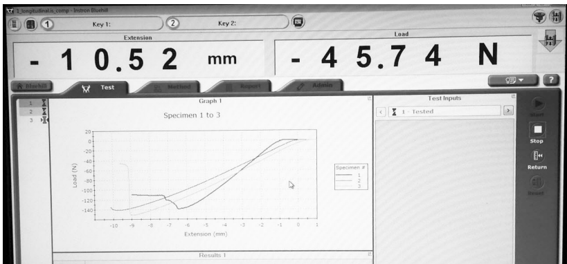
Graphs of load versus extension on the Heirloom laptop composite, as plotted by the Instron testing machine
