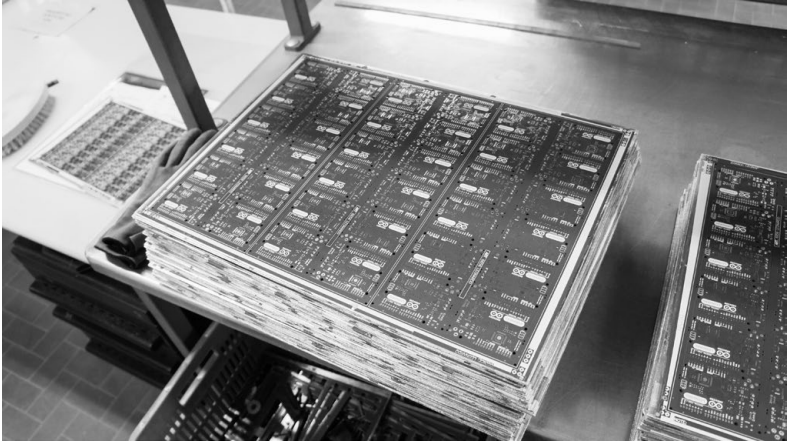
A stack of near-finished PCB panels, ready for a final step of routing out the individual boards
