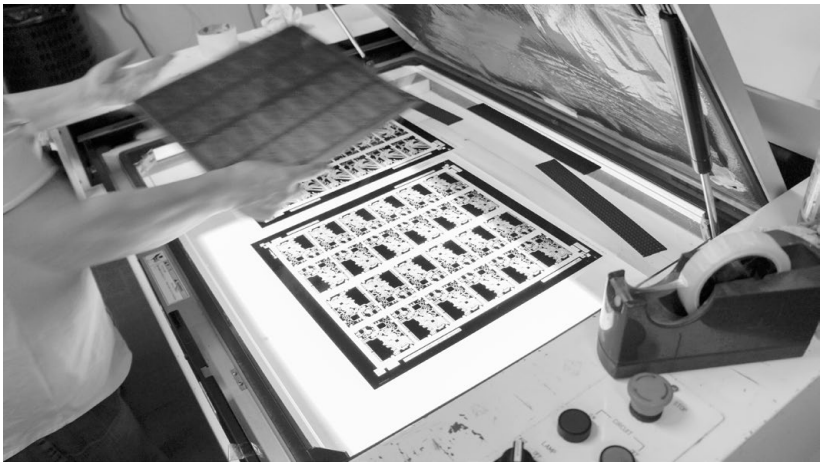
A PCB being mounted into a light box that will expose its unprocessed backside film
