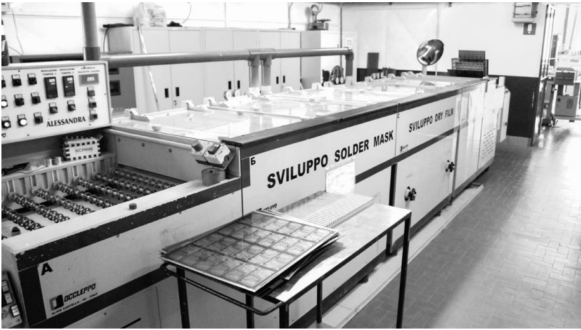
The machine that develops the photoresist
