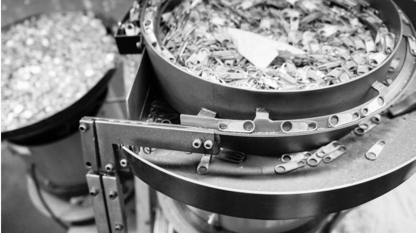
Pullers coming through the vibrapot
