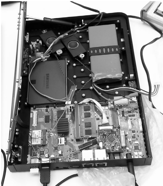
The T1 case base, in initial testing after the live hardware was transferred into the plastics
