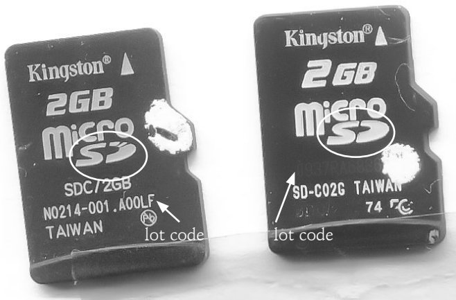
An irregular microSD card (left) and a normal card (right). The arrows and circles show suspicious differences.
