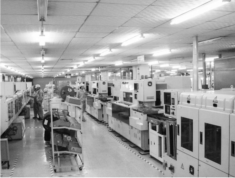
The chummy PCB assembly factory in China had dozens of lines filled with tried-and-true Fuji chip shooters.
