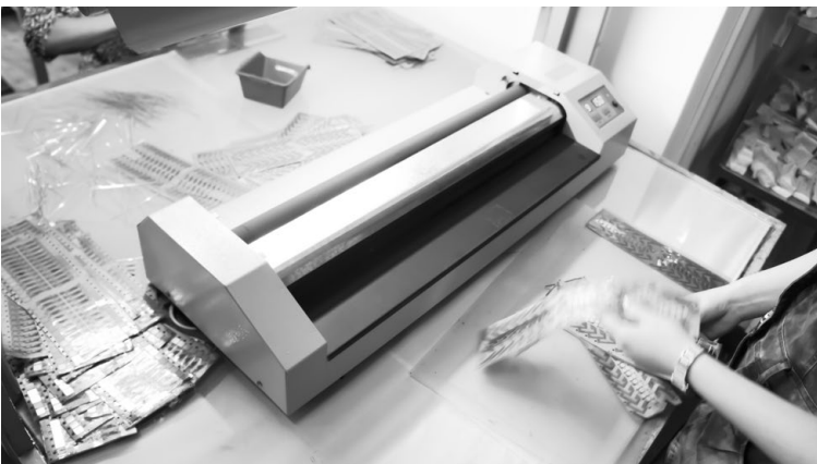
Steel plates being laminated to the back of flex-circuit material
