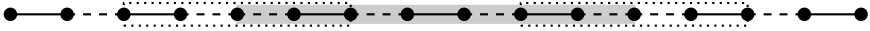
Fig. 6.1. An augmenting path (indicated by gray area) and environments of possible mutations leading to extensions or shortenings (dotted)
