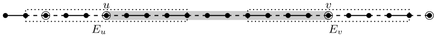
Fig. 6.2. An augmenting path (indicated by gray area) and the environments E_u and E_v (dotted); free vertices are indicated by a circle
