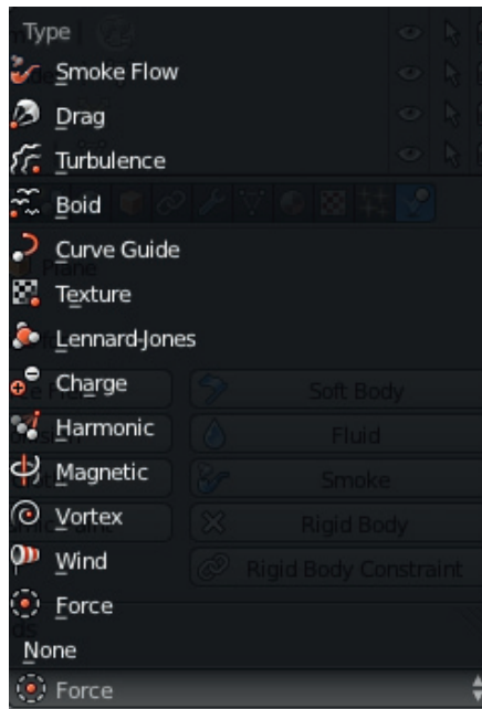
Figure 8.16. Fields available to the user with the Blender physics module. Mesh objects can be set to react to the physical constraints that occur because of a given field.
