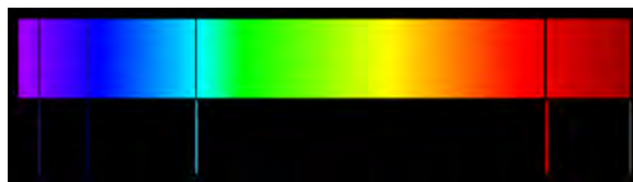
Figure 3.19. Top: an absorption spectrum. Bottom: the emission spectrum of the same element.
