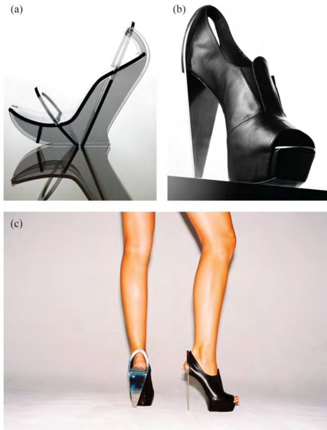
Figure 6.13. Shoes by Chau Har Lee. (a) Prototype flat packed shoe by Chau Har Lee made from seven pieces of Perspex which slot together and do not require glue. (b) and (c) retail version of shoe by Chau Har Lee with heel made from laser cut and welded stainless steel. (Photo (a) by George Ong and photo (b) by Sylvain Deleu. All photos courtesy of Chau Har Lee. Reproduced with permission.)
