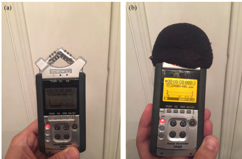
Figure 4.3. A pop shield reduces the air pressure reaching the diaphragm of a microphone when ‘p’ and ‘b’ sounds are spoken. These images show a Zoom H4N recorder which has a microphone at the top as seen in (a) when there is no pop shield in place. Image (b) shows the pop shield over the microphone. (© Julian Mayers. Reproduced with permission).
