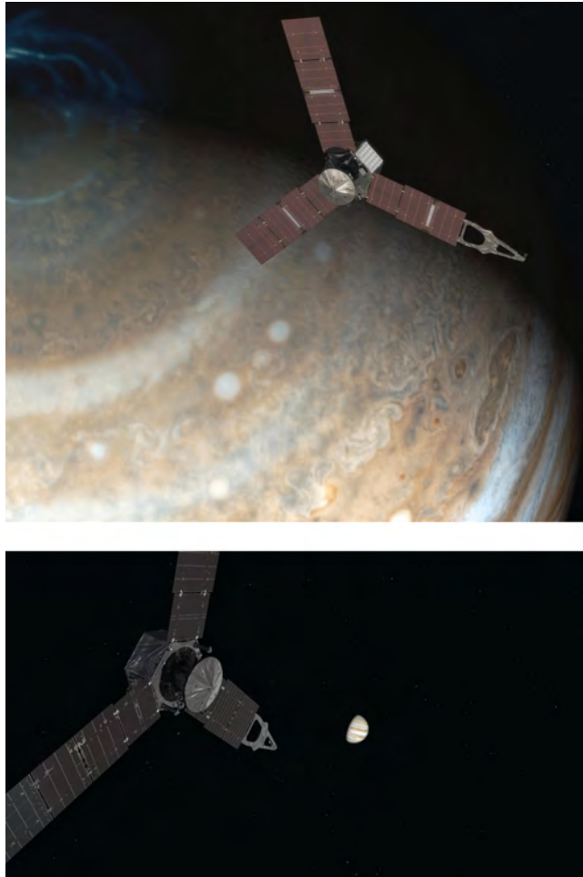
Figure 7.3. Artists impressions of the Juno probe near Jupiter, showing the three solar arrays. (a) Juno Above Jupiter's Pole (Artist's Concept). This artist's rendering shows NASA's Juno spacecraft above the north pole of Jupiter; (b) Juno Approaches Jupiter (Artist's Concept). This illustration depicts NASA's Juno spacecraft approaching Jupiter. (Image credit: NASA/JPL-Caltech).
