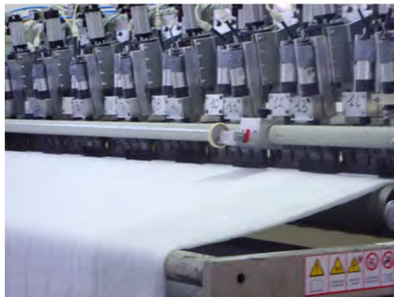
Figure 6.7. (a) Diagram showing the main parts of an ultrasonic welding machine; (b) an ultrasonic drum quilting machine. Outdoor jackets, for example, can be made from quilted fabrics. (Courtesy of TWI Ltd. Reproduced with permission.)
