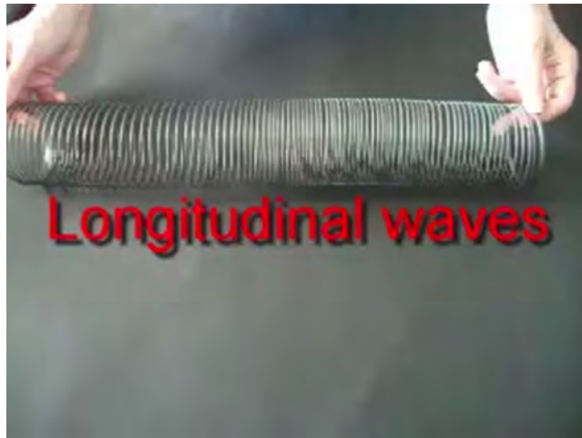
Figure/Video 4.1. Demonstrating the difference between longitudinal and transverse waves using a slinky spring and a skipping rope. To create longitudinal waves with a slinky spring one hand needs to remain still while the other hand is used to repeatedly push on the spring and so generate longitudinal waves that travel along the spring from one coil to the next. To create transverse waves with a skipping rope, one person needs to hold one end of the rope still while the other person moves their hand from side to side to generate transverse waves that travel along the rope towards the still end. (© Sharon Ann Holgate).
