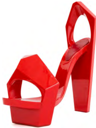
Figure 1.3. Resin shoe by Chau Har Lee made by 3D printing. (Photo by Charlotte Visser. Courtesy of Chau Har Lee. Reproduced with permission.)
