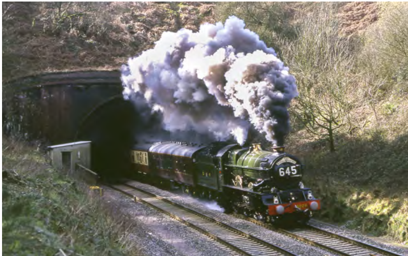
Figure 1.2. GWR King class locomotive (number) 6024 King Edward I in 1995 exiting the 1000 m long Whiteball Tunnel—which passes under the county border between Somerset and Devon in the UK, was designed by Brunel, and was built in 1844. Electronic safety equipment has been retro-fitted to this 1930s locomotive to enable safe running on the modern mainline. (© Martyn Bane. Reproduced with permission.)
