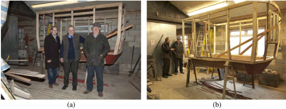
Figure 4.3. During restoration of Tony Drewitt's 1911 Garden-seat horse bus. (a) From left to right, Christopher Drewitt (Tony's son), wheelwright Edward Crouch owner of Croford Coachbuilders, and Tony Drewitt in front of the stripped down wooden bus frame. Edward, who is a Liveryman of The Worshipful Company of Wheelwrights, masterminded the restoration and together with his craftsmen stripped the body and wheels down, and made all the necessary repairs using the correct type of timber and working to some original plans of the horse bus construction; (b) side view of the shell of the bus with Tony and Edward discussing the project in the background. (© John Stiles. Reproduced with permission.)
