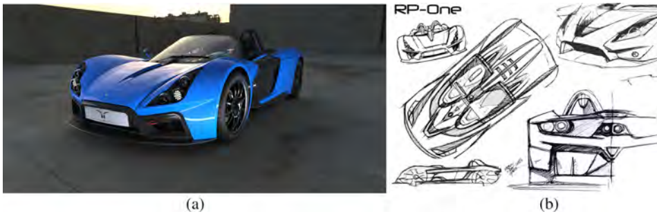
Figure 1.3. The Elemental Rp1 track day car. (a) The Rp1 has a carbon fibre tub, side pods, and dash panel, and thermoplastic composite Coats Synergex wheel arch liners. (b) These initial sketches of the Rp1 's bodywork by Guy Colborne were created after the ideas for the chassis and tub had been worked up in a CAD package. (© Elemental Cars Ltd. Reproduced with permission.)
