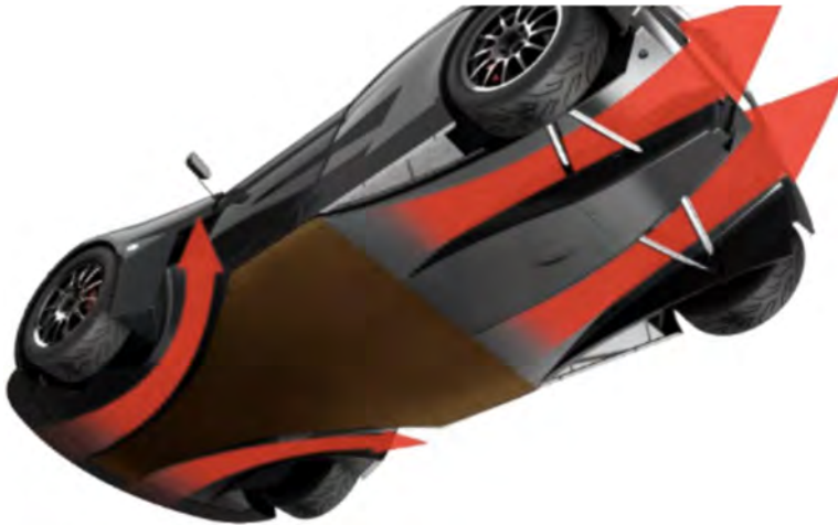
Figure 3.5. The air flow beneath the Elemental Rpl . (©Elemental Cars Ltd. Reproduced with permission.)
