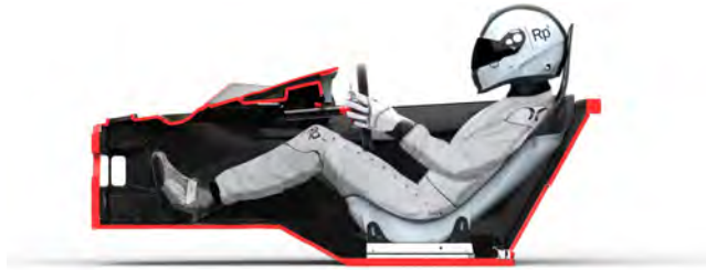
Figure 3.2. The feet-up driving position in the Elemental Rp1 . This feature is a first for a road car, and was defined by the positioning required for parts of the underfloor aerodynamics. (© Elemental Cars Ltd. Reproduced with permission.)
