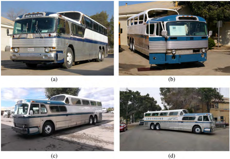
Figure 4.8. The Pacific Bus Museum’s 1955 Greyhound Scenicruiser, number 8005, at various stages of completion during its ongoing restoration. (a) Rust is visible on some of the bodywork in this picture taken in 2004, the year after the museum took ownership; (b) on static display in 2007 with restoration of the exterior underway; (c) pictured in 2014 with work on the body almost finished; (d) on the road in 2016 with the lining and logos completing the exterior restoration. (All images courtesy of Ron Medaglia. Reproduced with permission.)
