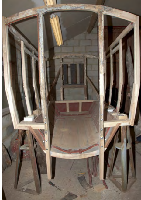
Figure 4.6. End view of Tony Drewitt's 1911 Garden-seat horse bus during restoration, showing the curved roof and upright posts. (© John Stiles. Reproduced with permission.)
