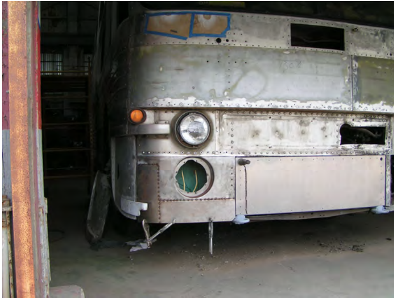
Figure 4.12. The wiring for 8005's headlights is visible in this 2007 image of restoration progress. The internal lighting, and the headlights and tail lights run off a 12 V circuit that is powered by a generator which in turn is driven by the engine. (Image courtesy of Ron Medaglia. Reproduced with permission.)
