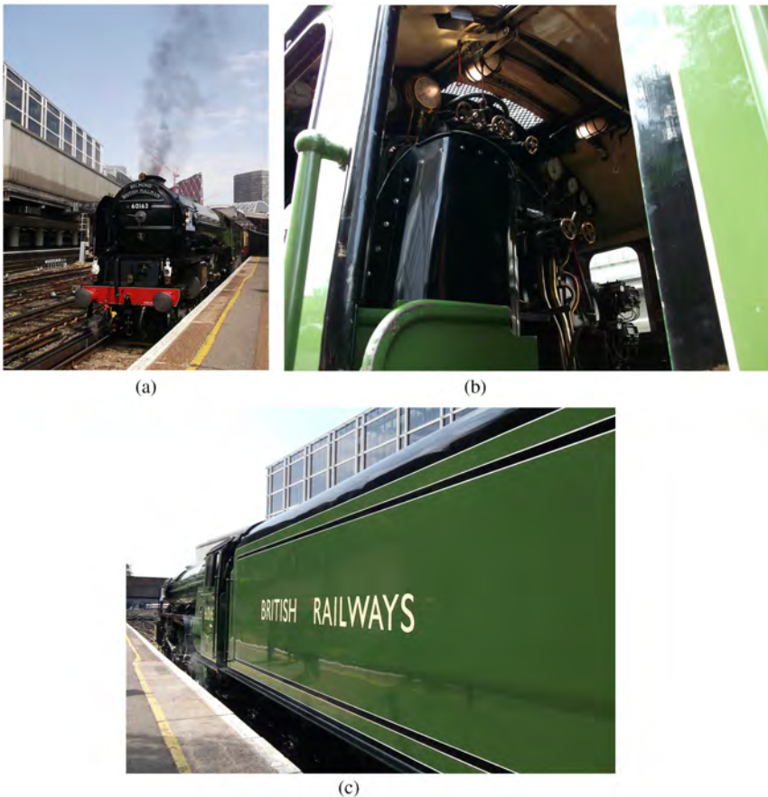
Figure 2.1. Tornado at Victoria station on Friday 27 May 2016 about to depart with a Belmond British Pullman excursion; (a) front view, (b) inside Tornado 's cab: the driver's seat is shown on the left-hand side; (c) view showing Tornado 's tender, which can carry 7.6 tonnes of coal, and approximately 27 276 litres (6000 gallons) of water. This gives the locomotive a range of around 161–177 km (100–110 miles) before needing to take on extra coal and water. (© Sharon Ann Holgate, 2016.)
