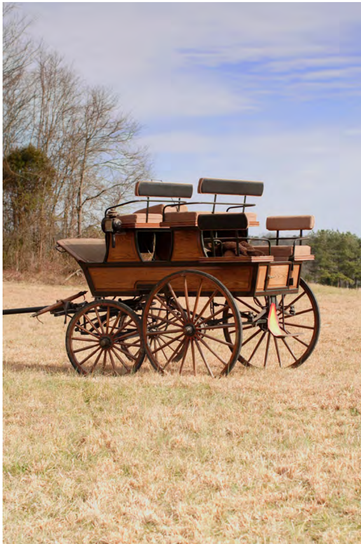
Figure 4.5. An American horse-drawn buggy. Designs like this influenced the wheel design for horse buses in the UK. (© DESmith Photography/Shutterstock.com.)
