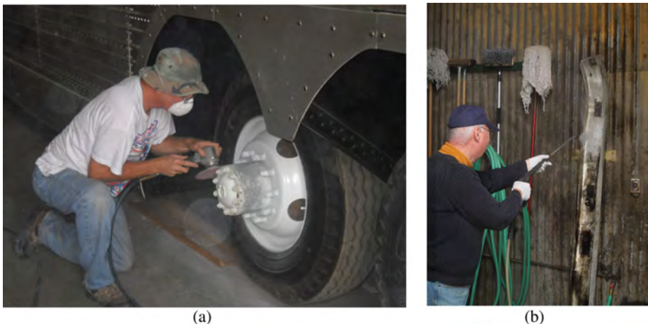
Figure 4.11. Modern power tools helped speed up the restoration process. (a) Here Pacific Bus Museum volunteer Mitch Roberts is using an air powered sander to sand the wheel hub before it is repainted; (b) Pacific Bus Museum volunteer Homer Beaudoin cleaning dirt off 8005’s rear bumper using a portable gasoline powered pressure washer that pressurizes water through a tip at 2500 psi (17 240 kPa). (All images courtesy of Ron Medaglia. Reproduced with permission.)
