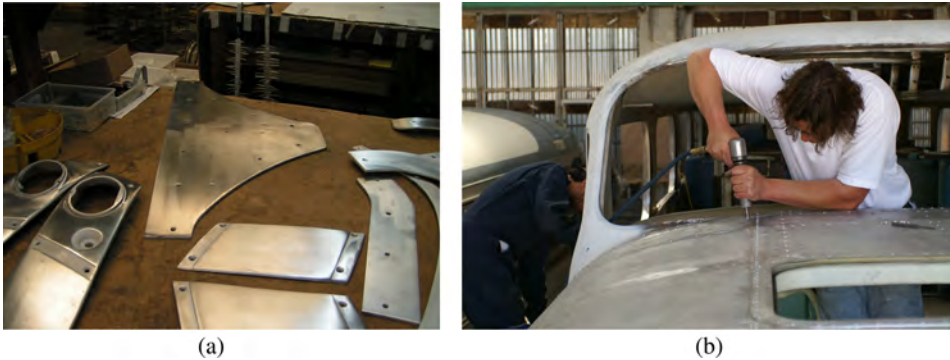
Figure 4.10. Greyhound Scenicruisers have an aluminium and steel monocoque construction. (a) Shows re-conditioned exterior trim pieces from bus 8005. Each piece was first chemically stripped and cleaned, before being belt sanded with 600 grit sandpaper to remove any scratches and restore the original ‘brushed’ finish. The pieces were then re-anodized in a clear aluminium anodizing solution; (b) Pacific Bus Museum volunteer Mike Browne bucking a rivet using an air powered rivet gun on a replacement panel on the upper windshield. (All images courtesy of Ron Medaglia. Reproduced with permission.)
