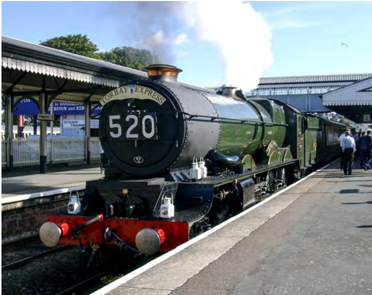
Figure 2.15. Locomotive 6024 King Edward I at Paignton in Devon. Pictured on the right of the photograph at the front of the locomotive is a battery-powered headlamp with a halogen bulb. This is fitted inside the casing of a portable vintage oil lamp similar to the lamps the locomotive would originally have used. A traditional paraffin lit lamp is on the left of this photograph. The two lamps to the side, sitting up on the running plate, are spares which were traditionally carried in that position. (© Martyn Bane. Reproduced with permission.)
