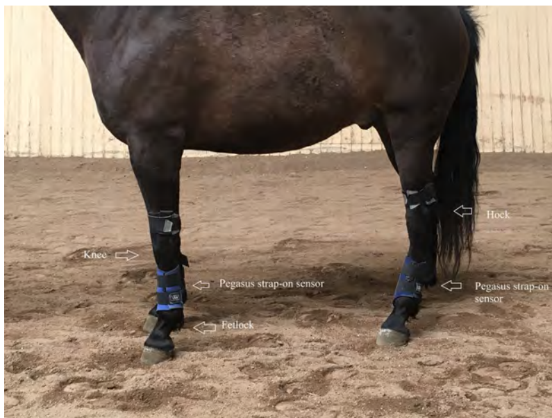
Figure 4.7. Eight Pegasus sensors strapped onto a horse’s legs ready for carrying out a gait analysis. Each sensor contains an IMU. (© Diana Hodgins. Reproduced with permission.)
