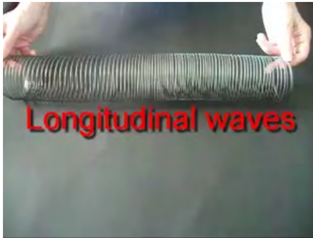
Figure/Video 4.4. Demonstrating the difference between longitudinal and transverse waves using a slinky spring and a skipping rope. To create longitudinal waves with a slinky spring one hand needs to remain still while the other hand is used to repeatedly push on the spring and so generate longitudinal waves that travel along the spring from one coil to the next. To create transverse waves with a skipping rope, one person needs to hold one end of the rope still while the other person moves their hand from side to side to generate transverse waves that travel along the rope towards the still end. (© Sharon Ann Holgate.) Video available at https://iopscience.iop.org/book/978-1-64327-670-0 .
