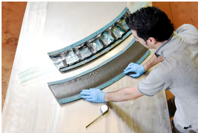
Figure 2.18. Creating a carbon fibre component for a racing car. (© fabiodevilla/Shutterstock.com).
