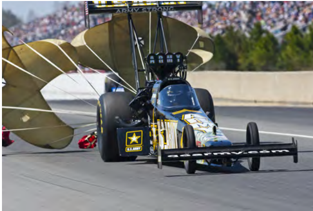
Figure 3.6. Driver Tony Schumacher slows his Top Fuel race car during the Tire Kingdom NHRA Gatornationals race at the Gainesville Speedway in Gainesville Florida USA on March 12th 2011. The deployed parachute helps bring the race car to a halt. (© Action Sports Photography/Shutterstock.com.)
