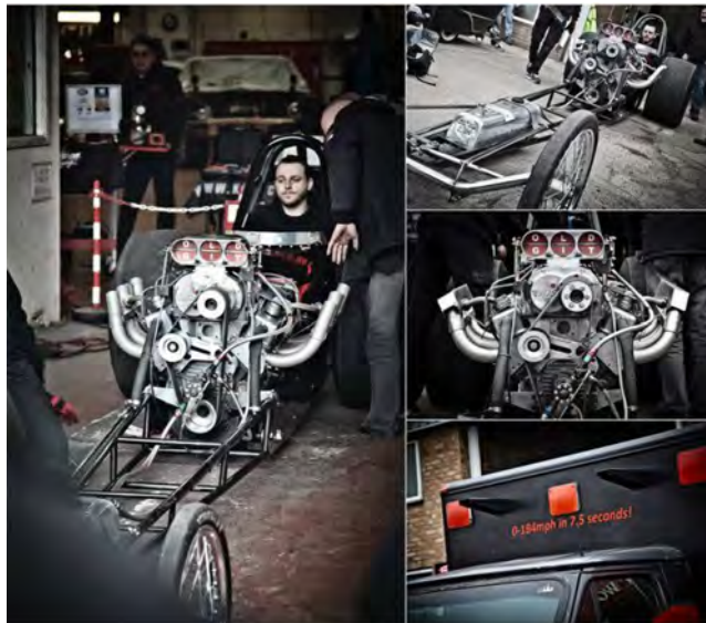
Figure 3.4. Views of Alec Coe’s dragster. The three round flaps emblazoned with ‘Old Git’ let air into the engine. (© Alec Coe. Reproduced with permission.)
