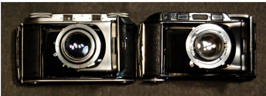
Figure 3.18. The lens on the left (from the 1950s) is single coated, while the even-older lens on the right is uncoated. Note the slightly-purplish and much-fainter reflections from the coated lens.
