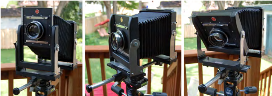
Figure 12.4. Front movements on a 4 \times 5 monorail view camera. Left: front rise. Center: front right swing. Right: front forward tilt.
