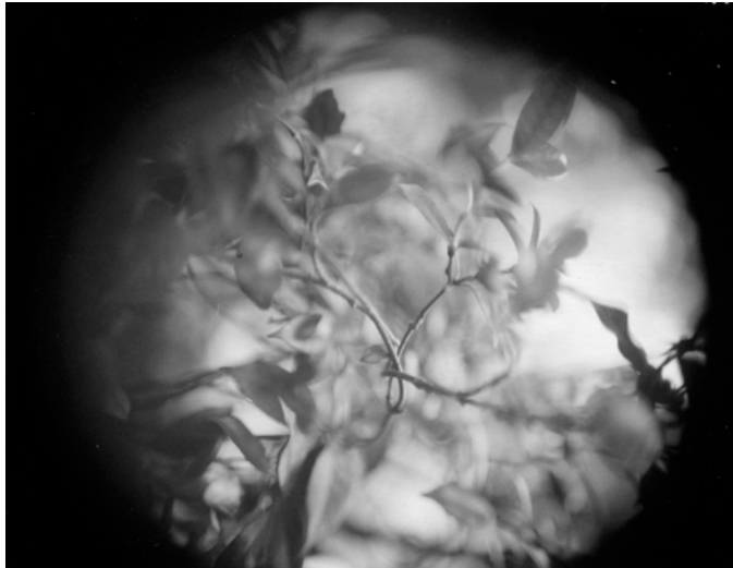
Figure 12.5. An example of a picture taken with a lens that does not cover the particular film format used. The image circle is smaller than the film, and the picture shows pronounced vignetting.
