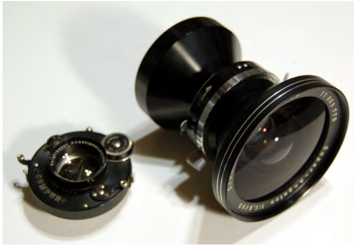
Figure 12.7. Left: 114 mm f/4.5 Voigtländer Anastigmat Skopar. Right: Schneider 90 mm f/5.6 Super Angulon. Even though the Skopar on the left has an aperture that is physically over 50% larger, the lens is much smaller and lighter. This is because the Super Angulon on the right is better corrected for aberrations, and has a much larger image circle . The Skopar was meant to cover film with a diagonal of only 5" (58° angle of view), without movements. The Super Angulon, on the other hand, has an image circle of 9.25" with a 105° angle of view. This allows it to easily cover 4 × 5 inch film with room for substantial movements.
