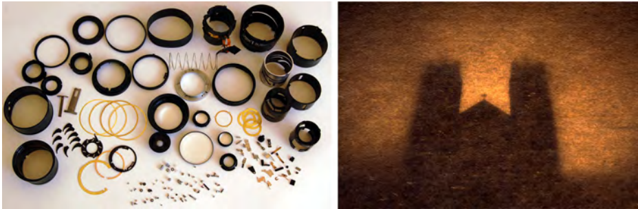
Figure 9.15. Left: a modern camera lens contains many lens elements and precision moving parts. Right: St. Mary's Church . John Beaver 2003. This picture was taken with only a simple double-convex lens.
