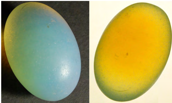
Figure 3.13. Tyndall-effect scattering in an egg-shaped piece of opalescent glass. The photo on the left was taken with the egg against a black background and illuminated from above. We see the mostly-blue light that is scattered back towards us. The photo on the right was taken with the egg illuminated from behind. In this case we see the light that was not scattered by the egg on its way to us. Since mostly blue light is scattered, what is left over appears reddish in color.
