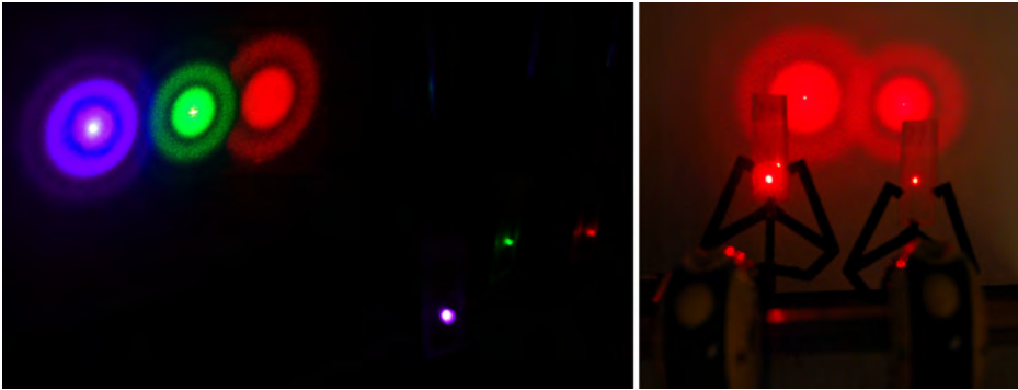
Figure 3.21. Left: lasers of three different wavelengths shine through smears of human red blood cells. The diffraction pattern is large because the cells are so tiny. The central portion of the bulls-eye pattern is smallest for the violet (short wavelength) light and largest for the red (long wavelength) light. Right: two lasers of the same wavelength shine through different smears of red blood cells. The diffraction pattern on the left appears slightly larger because the smear was made with red blood cells from a dog, and they are slightly smaller than the human red blood cells used on the right.
