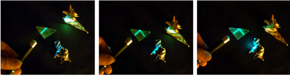
Figure 3.9. A 45° glass prism used to reflect light by 90°. Left: the light meets the backside of the prism at less than the critical angle. It mostly passes through, deflected by refraction. Notice, however, that a small portion of the light reflects off the surface internally, like a mirror. Center: the light meets the back face of the prism at very nearly the critical angle, and refracts almost parallel to the back face of the prism. Notice that the internally reflected portion is now much brighter. Right: the ray meets the back surface at greater than the critical angle, and all of the light reflects internally.
