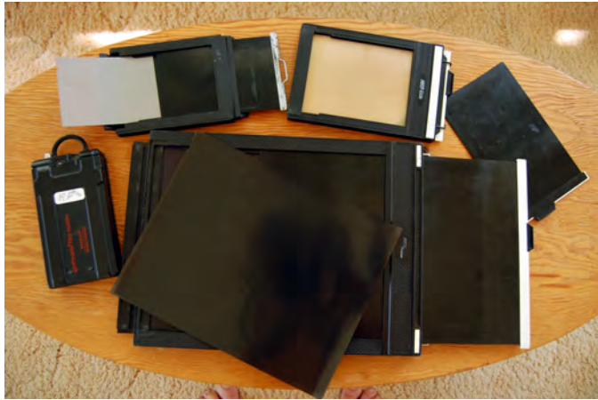
Figure 12.3. Examples of film holders for different formats of sheet film. Clockwise from upper left (all sizes in inches): 3\frac{1}{4} \times 4\frac{1}{4} film holder, with sheet film partially inserted; 4 \times 5 holder with film loaded; dark-slide cover for the 4 \times 5 holder; 8 \times 10 film holder with dark slide and sheet of film; a special 'graphmatic' 2\frac{1}{4} \times 3\frac{1}{4} holder that can hold six sheets of film, with an internal mechanism to allow rapid shuffling from an exposed sheet to the next unexposed sheet.
