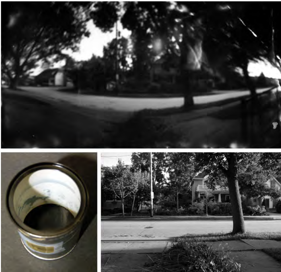
Figure 12.13. Top: this ephemeral process pinhole image was made with the light detector curved around the inside of a cylinder. Bottom left: the pinhole camera, with the just-exposed negative in place. The pinhole can be seen as the small piece of brass on the front of the cylinder. Bottom right: the same view as imaged with an ordinary wide-angle lens. The pinhole camera made a wider view, and the straight street seems to bend.
