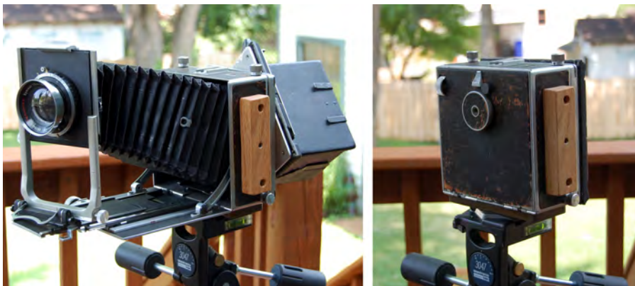
Figure 12.2. A vintage German-made Linhof Technika III technical camera , that uses 4 \times 5 inch sheet film. This particular example was originally made in 1950, but it has had some recent modifications. A technical camera has many, but not all, of the same movements (left image) found on a monorail. Others can be ‘faked.’ But unlike a monorail, a technical camera folds up (right image) into a small box. A field camera (not shown) is similar, but made of wood, somewhat bulkier but lighter and yet more rugged, and usually with more limited movements than a technical camera.
