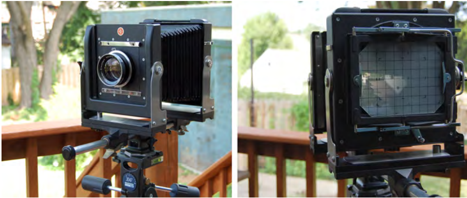
Figure 12.1. A monorail view camera that uses 4 \times 5 inch sheet film. The lens is attached to a front standard while the focus screen and film are mounted on a rear standard . Both are attached so they can slide along a rail, and a flexible bellows keeps light out. This arrangement allows for standards that can accomplish a wide variety of movements (section 12.1). The image to the right shows the ground-glass focus screen. On this particular monorail the entire focus screen can rotate in order to accommodate both portrait and landscape formats without needing to tilt the camera itself.
