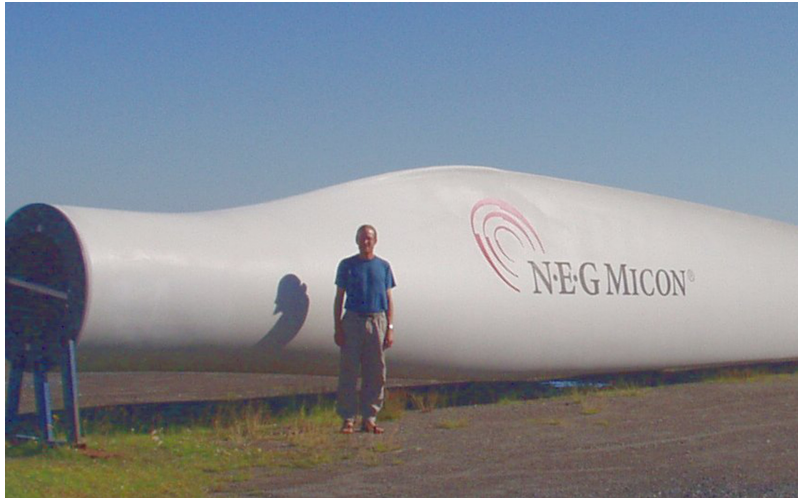
Figure 6.4. A single wind turbine blade, 20 m long, from a small wind turbine. (Photograph taken by the author.)
