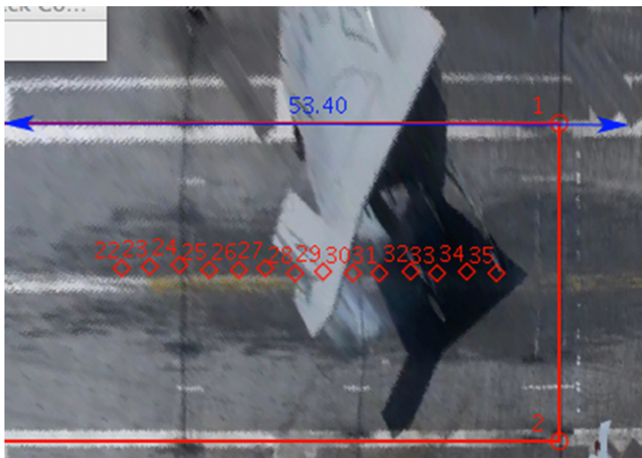
Figure 4.5. Screen capture from Tracker Video Analysis (Software made available under the GNU General Public Licence, version 3 (GPL-3.0).) showing the marked locations of a drone as it lands. This is based upon [1].
