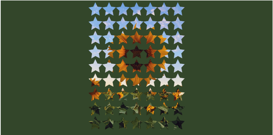
9-29. Setting the mask-size property means that it can repeat more often across each dimension
