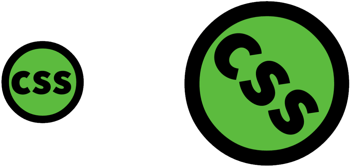
8-18. The original element (left) and after a combined rotation and scaling transformation is applied (right)
