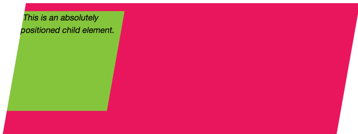
8-5. A child element with position: absolute nested within an element with transform: skewX(-15deg)
