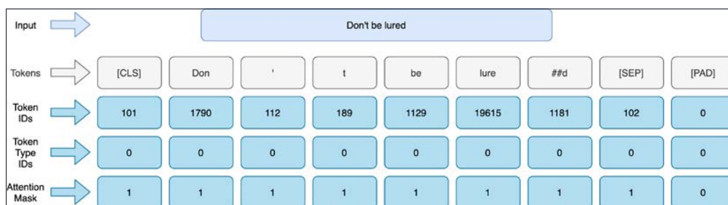
Figure 4.7: Mapping inputs to BERT sequences
