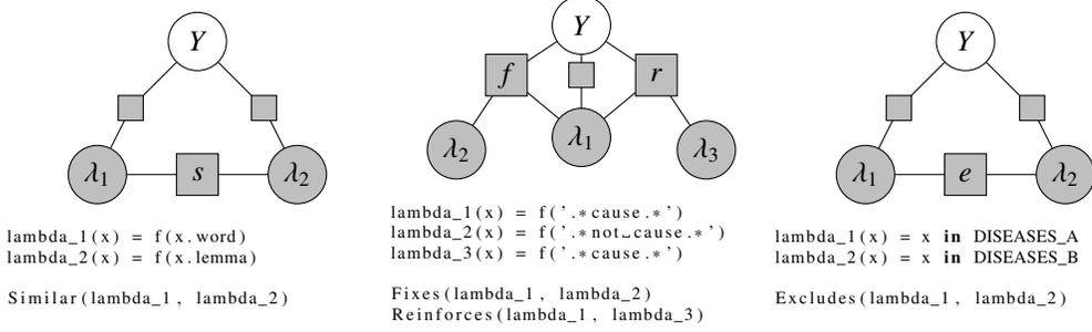
Figure 2: Examples of labeling function dependency predicates.
