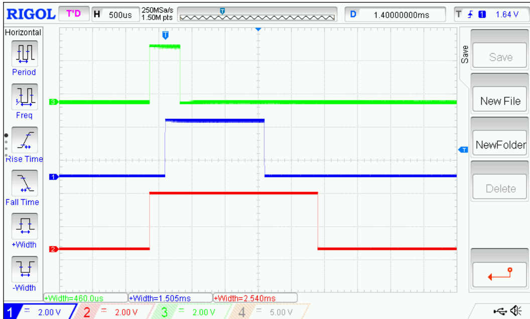
Figure 18.15: The same three servos, but with the signal zoomed in and the bottom legend switched to timings
