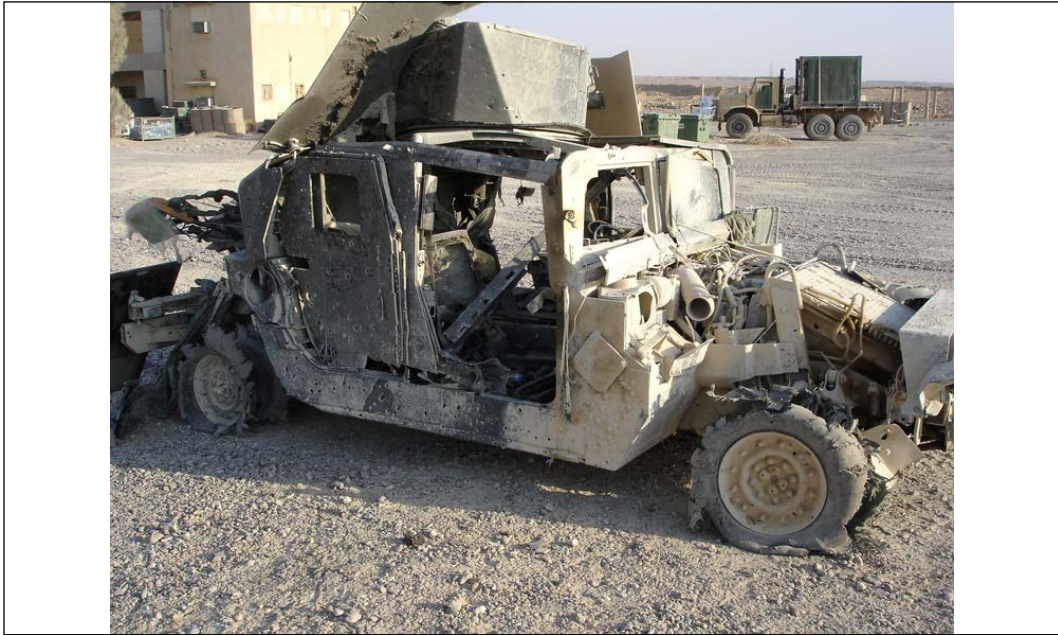
Figure 2: The damage that a Humvee sustains from an IED thanks to its light armor
