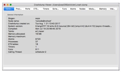
In the crash dump, you'll find information about running processes, ports, ETS tables, atoms, modules, memory usage, and more. You can tell exactly how the crash happened. If a system terminates for an unknown reason, the crash dump alongside the log and SASL reports we enabled earlier in this chapter should provide enough data to isolate the issue to a specific part of your application.
