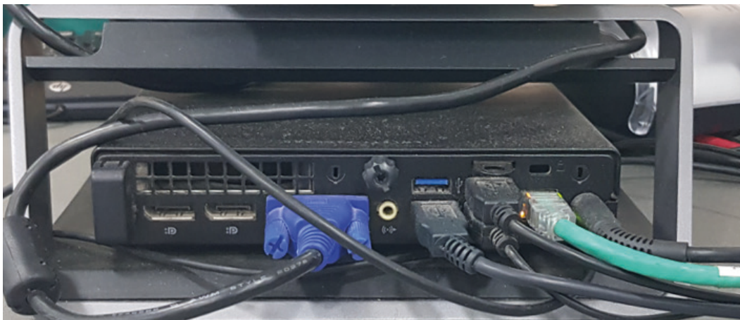
Figure 2.10 – Small form factor PC with one exposed USB port facing the customer
