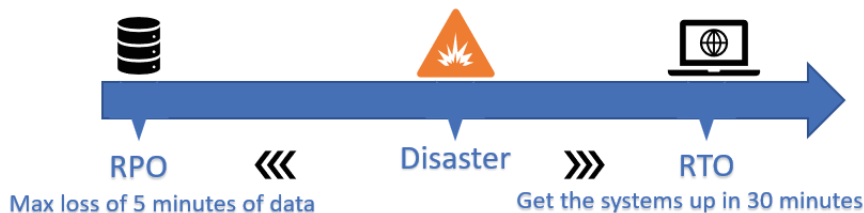
Figure 2.17 – An example of RPO and RTO
