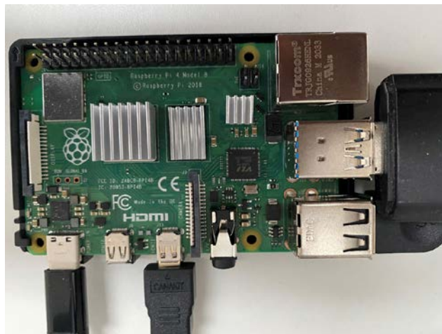
Figure 5.8: Photo of assembled Raspberry Pi 4
