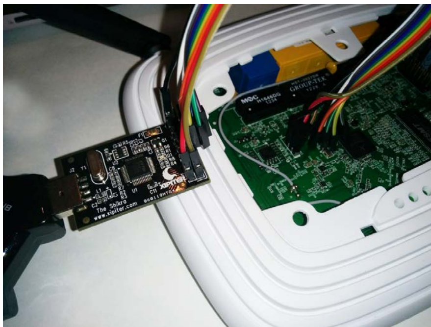
Figure 14.12: Connecting the UART to Cisco Meraki MR18 wireless access point
