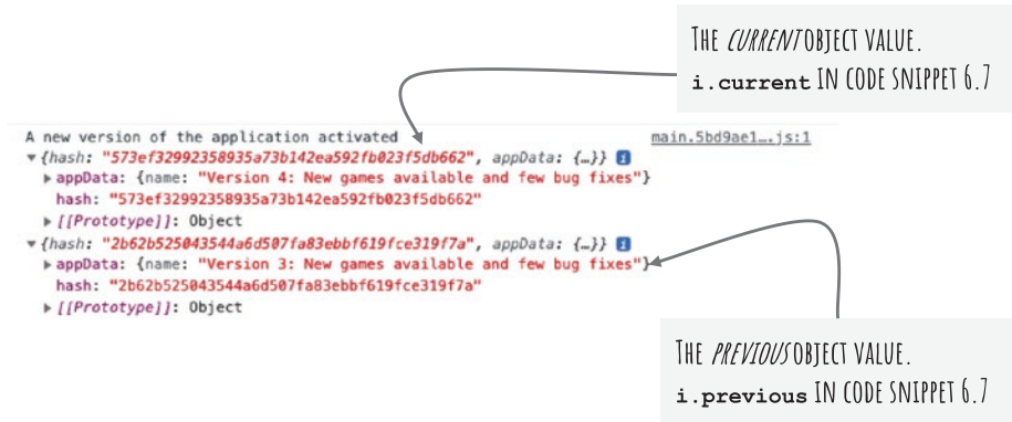
Figure 6-2. Result on the activated observable
