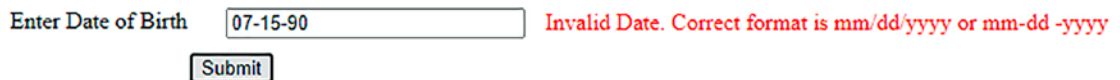
Figure 4-11. The error message Invalid Date is displayed if the date is entered incorrectly
