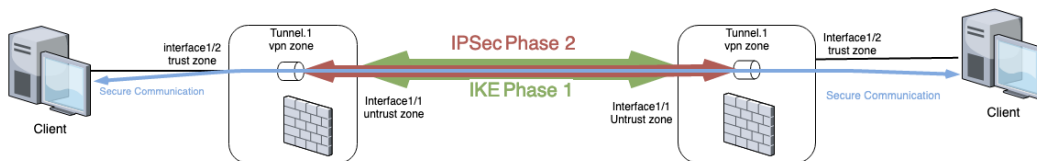
Figure 10.6 – A VPN tunnel from the firewall's perspective
