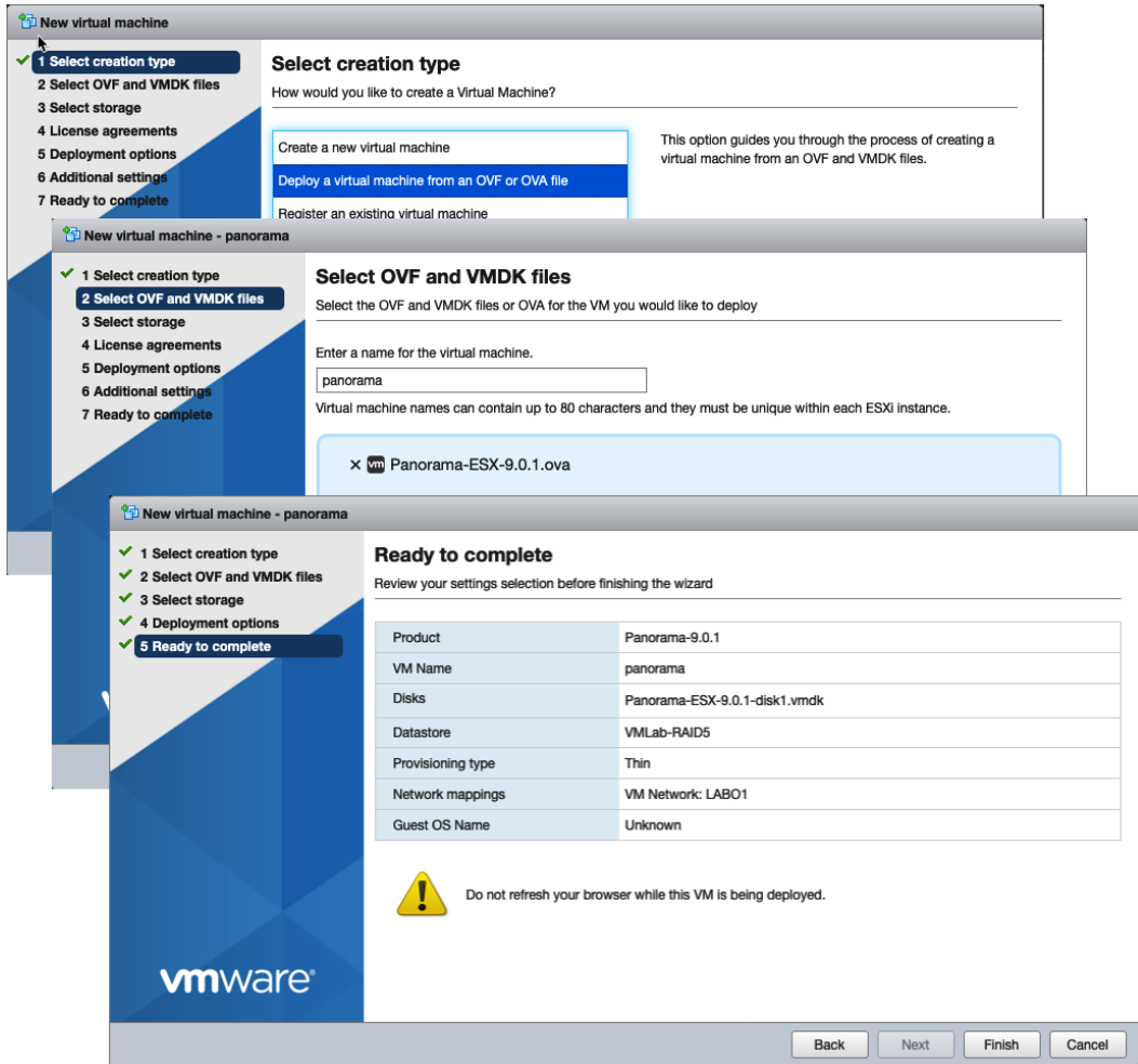
Figure 7.1 – Deploying a Panorama OVA in ESXi
