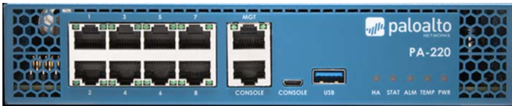
Figure 2.2 – PA-220 RJ45 and the micro USB console ports
