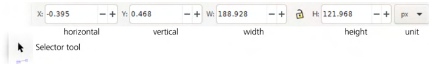
Figure 6-10: The Selector tool's controls bar: the X, Y, W, and H fields
