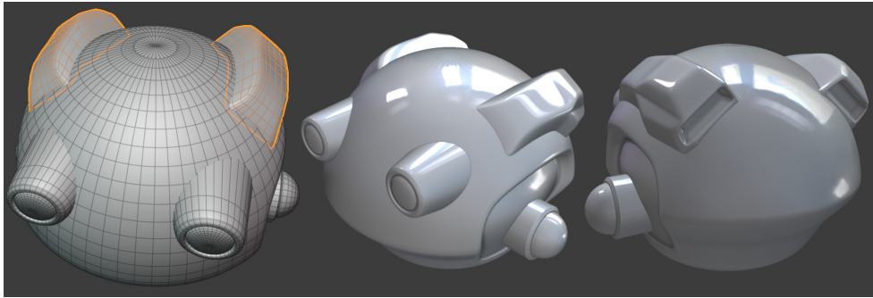
Figure 2.35 – The Booster_V1 model placed on the body and mirrored to the other side
