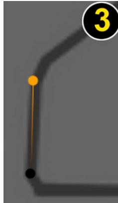
Figure 2.44 – Extruding the vertex to create edges that follow the outline of the claw
