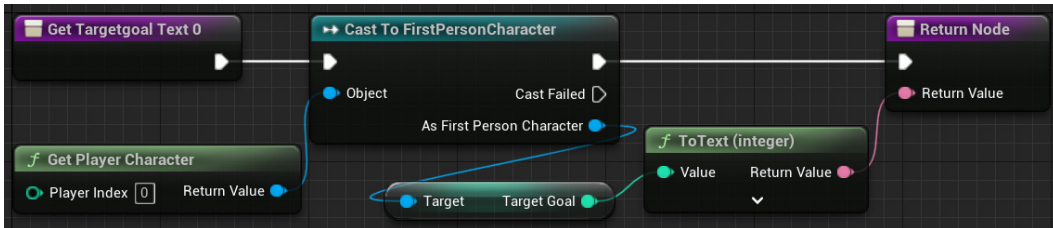
Figure 8.29 – The value of the Target Goal variable will be shown on the HUD
