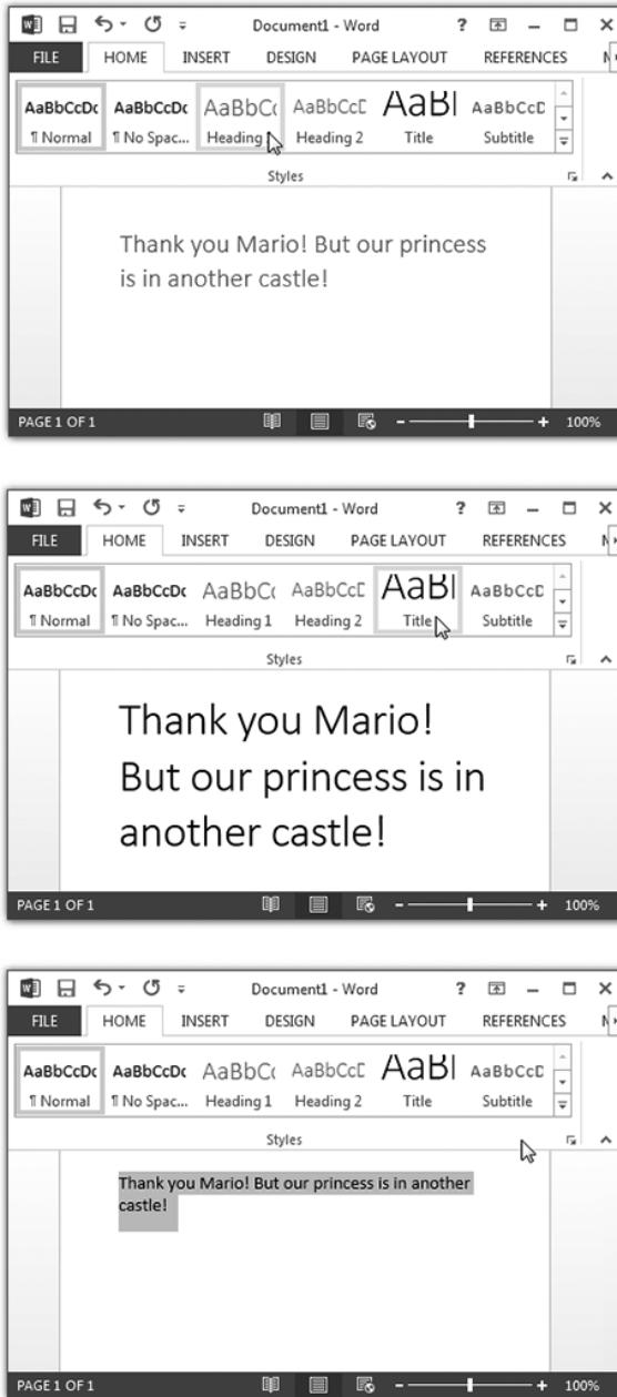
FIGURE 5.23 Using feed-forward to preview changes to formatting in Microsoft Word. Used with permission from Microsoft.
