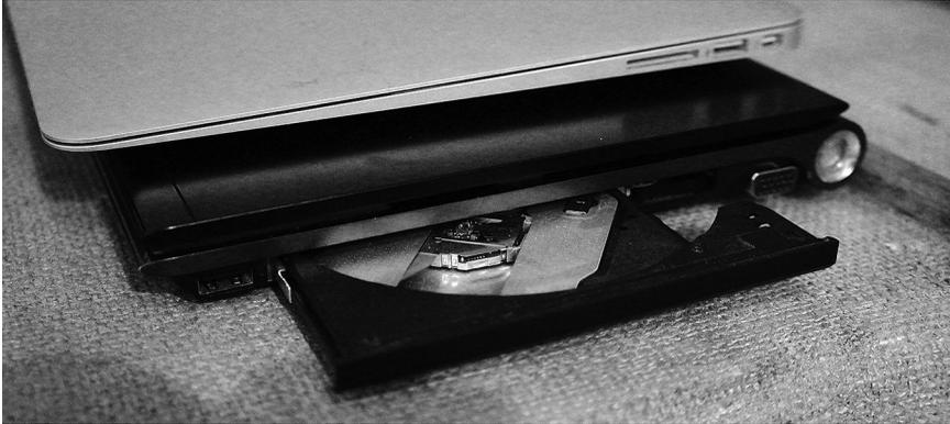
FIGURE 3.6 While other manufacturers were constrained with the assumption that all laptops must have a disc drive (bottom), Apple observed that very few people used their laptop disc drives, and decided to use that space to make a thinner laptop with better battery life (top).
