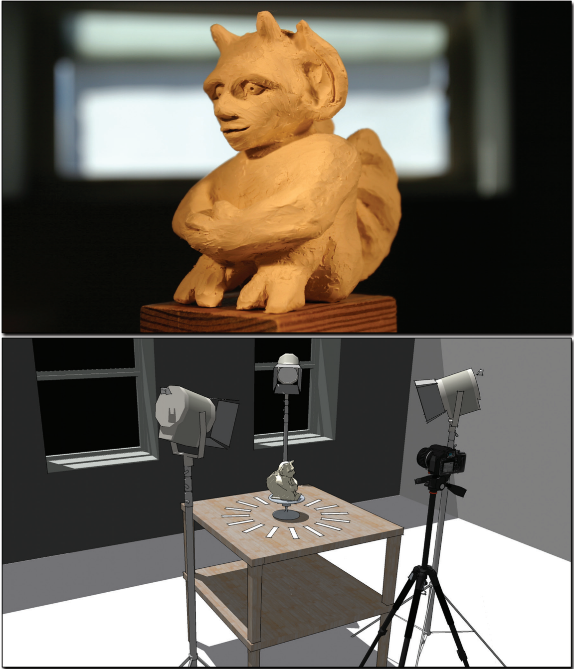
FIGURE 7.9 Studio setup for mesh capture with sample photo of the gargoyle sculpture created during the process. Studio equipment models are from the SketchUp 3D Warehouse.
