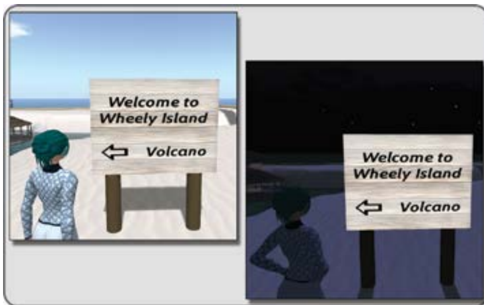
FIGURE 5.15 Screen shot in OpenSim showing a sign with “Design for All” considered in its construction. This is readable by most vision types. The front face is set to full bright so that the sign is visible even in a night setting.
