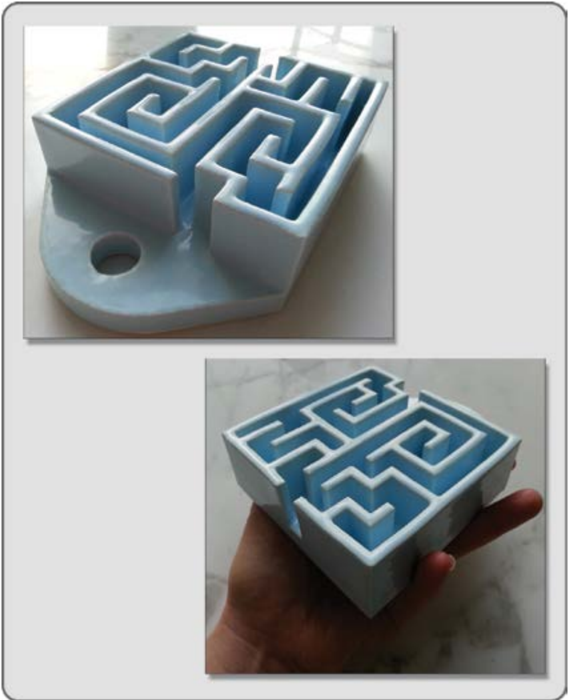
FIGURE 13.19 Photo of maze model, created as a physical world prototype printed out of a ceramic material by Shapeways.
