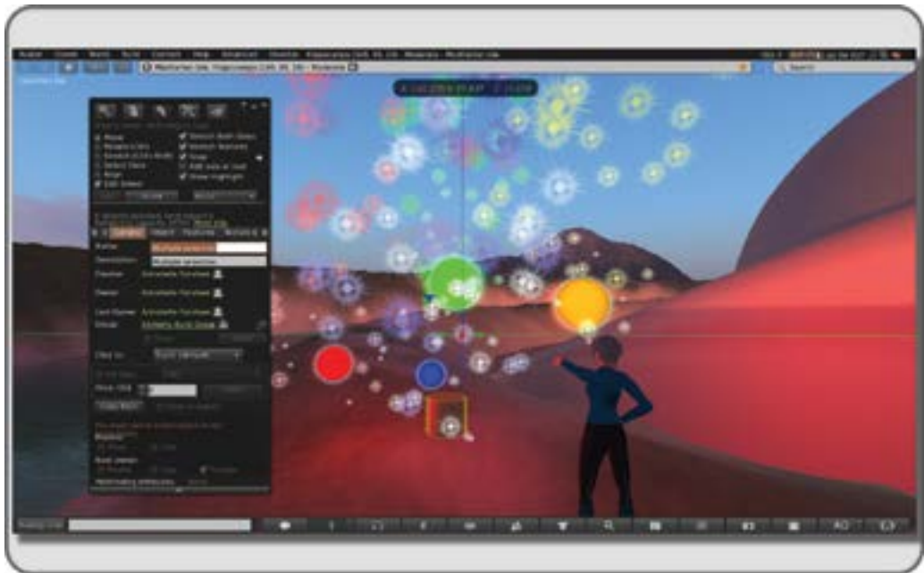
FIGURE 7.9 Screen grab showing result of making the particle emitting prims into light sources, coloring their texture, and linking them to the central cylinder.
