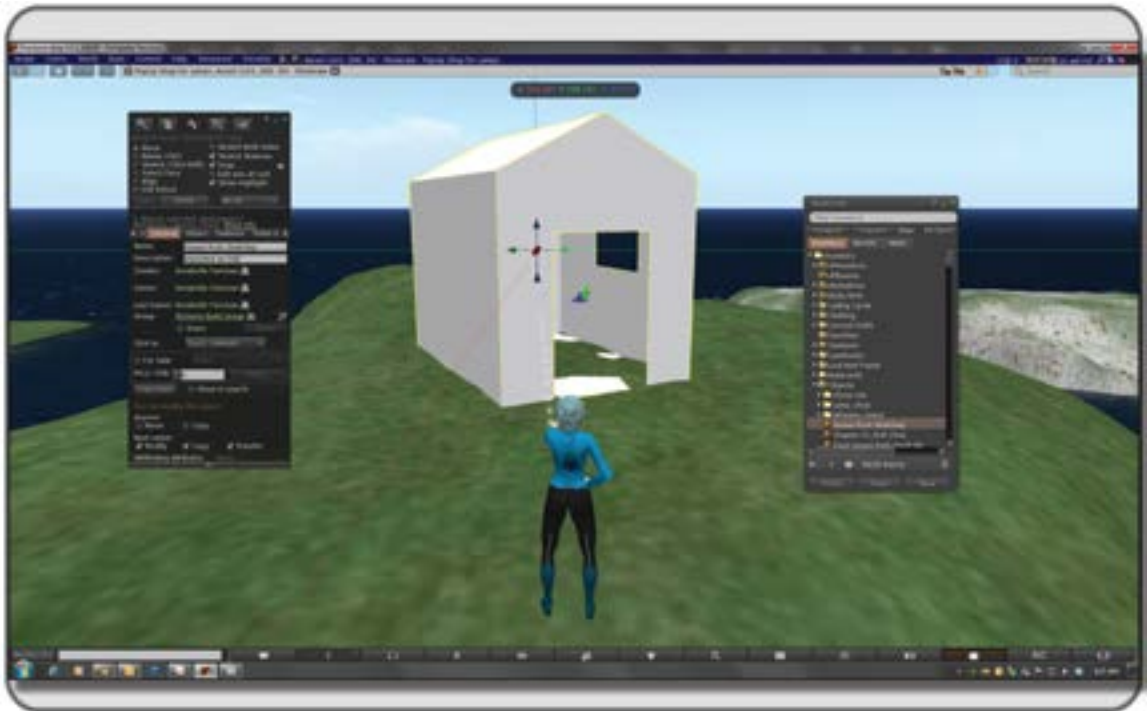
FIGURE 3.13 Screen grab showing the SketchUp house model (saved as a COLLADA (.dae) file) after it has been uploaded into OpenSim.
