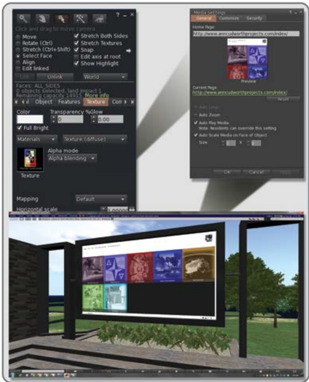
FIGURE 9.9 Screen shots showing an overview for installing media on the surface of the Ideagora. In the top left image, the Build/Texture tab menu in the Firestorm Viewer showing Media Channel Reminder texture and Materials setting. In the top right image, the secondary menu under the Texture tab, which is a dropdown menu from the Materials button, allows for Media to be assigned to any surface with a designated media texture. In the bottom image, the media screen displaying the designated web page on its surface.
