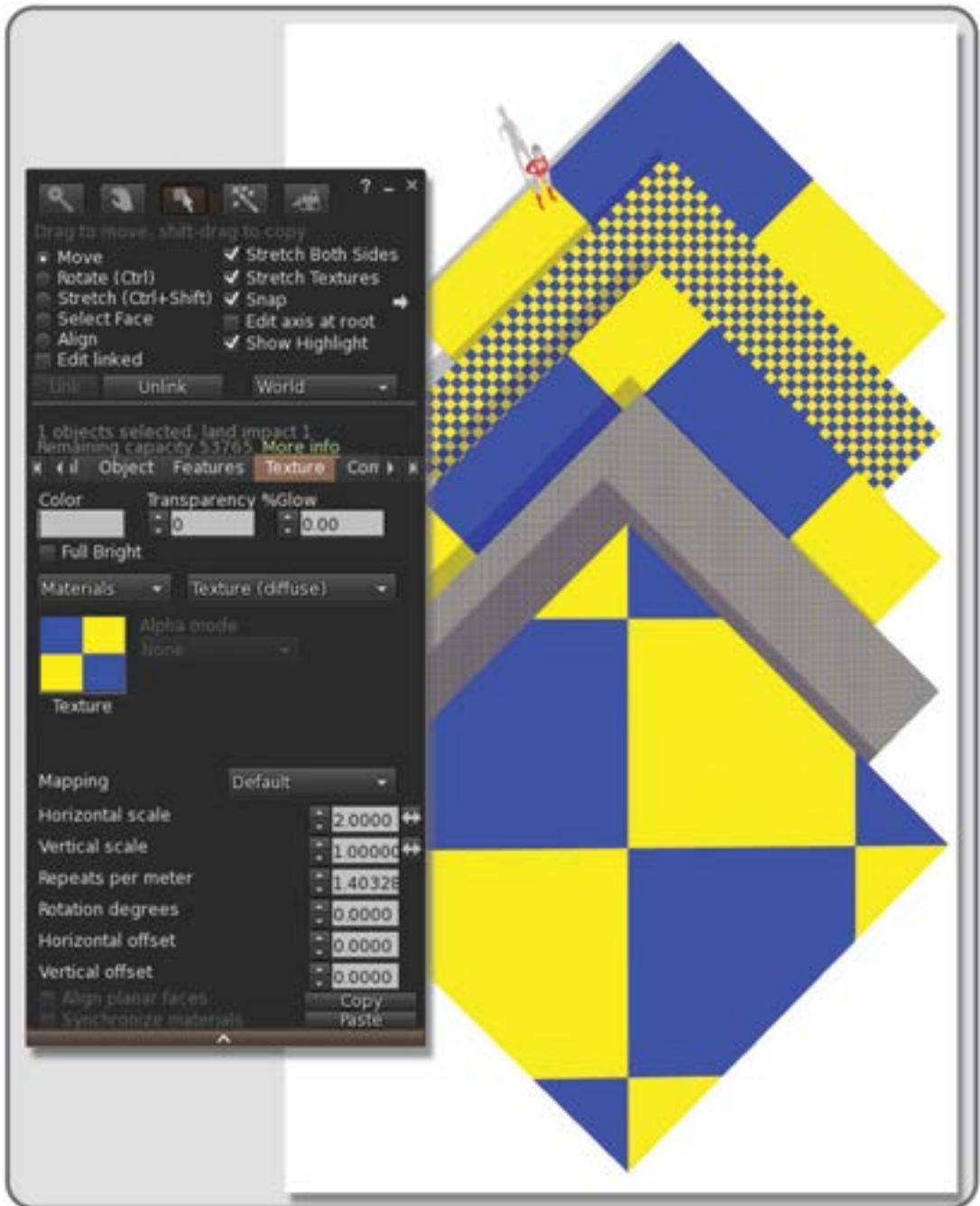
FIGURE 6.16 Screen grab from OpenSim, showing various ways to tile a single texture on a 10 m square prim. From the top down on the right, these modifiers are shown: default, planar, offset on the U and V, 10 repeats/meter, and rotation of texture 45 degrees. On the left is the texture tab of the Build menu, tiling options for textures are in the lower section.
