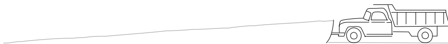
Fig. 65. Cross-section, showing the varying height of snow in front of the plow when the system is in its steady state.
