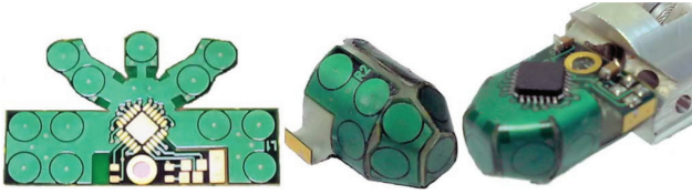
Figure 1.2 E-skin on iCub fingertips. From [1]. Reprinted with permission from IEEE.
