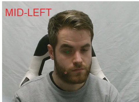
Figure 7.5 Eye gaze system results: the pupil position (green circle), calibration point (red point), and gaze area estimation (red text).
