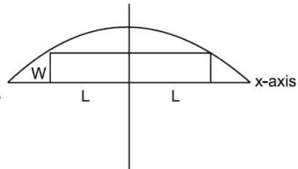
$$\frac{d^2A}{dL^2} = -12L \Rightarrow \text{at } L = 2 \Rightarrow \frac{d^2A}{dL^2} = -12 \times 2 = -24 < 0 \Rightarrow \text{Max}$$
