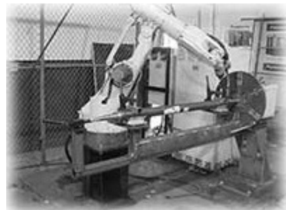
FIGURE 11.7 Robot Performing Sealing Operation
