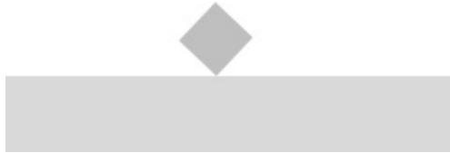
Figure 2.21: A block at tipping point
