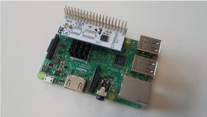
Figure 4.5 Raspberry PI model 3 with TPM dedicated hat in white.
