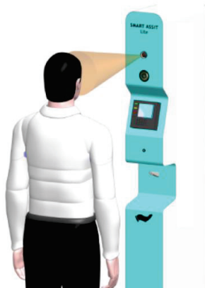
Figure 4.4 A smart assist kiosk monitoring mask wearing, thermal screening, and automatic sanitizer dispensing [12].
