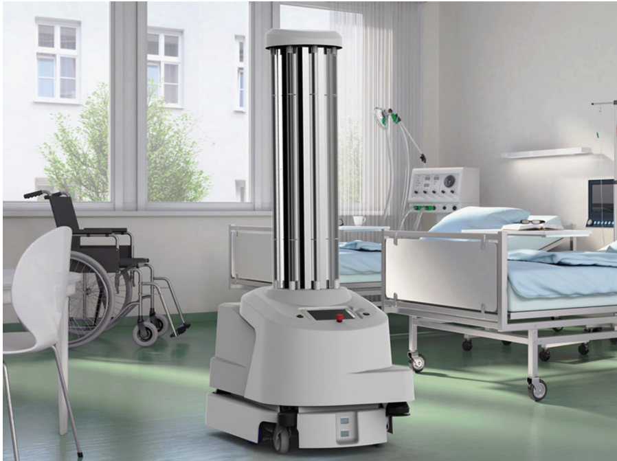
Figure 5.2 TurtleBot UV disinfectant robot.
