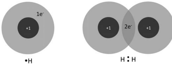
FIGURE 1.8: The covalent bond in its simplest form between a pair of H atoms to form the H_2 molecule.
