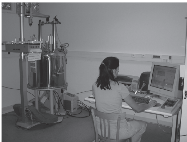
Figure 4.14 The dream of the NMR quantum computer: A hot water tank–looking NMR spectrometer of the type typically used in NMR quantum computing. The vial of molecules in solution to be used as the qubits is loaded into the port at the top. The bulk of the tank consists of strong magnets whose magnetic fields are used to align the spins of the nuclei in the molecules. The other metallic things sticking out of the tank are the radio wave pulse generators that are used to manipulate the qubits via a computer console off to the right. It was so simple it seemed to be too good to be true and it was. (Photograph of an NMR spectrometer by Daniel Alexandre [March 28, 2008].)
