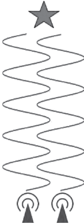
Figure 4.11 Two phased radar antennas (triangles) radiating at a single target (star). The antennas are coherently phased so that the electromagnetic radar waves (wiggles) are perfectly in sync. That is, the waves' peaks and troughs line up peak to peak and trough to trough. The rule of coherent addition of radio waves tells us that the radar power at the target, I_{\text{two antennas}}^{\text{coherent}} = (1 + 1) \times (1 + 1) = (2) \times (2) = 4 , is double than it would be from the two antennas if there were no coherence, I_{\text{two antennas}}^{\text{coherent}} = (1+1) \times (1+1) = (2) \times (2) = 4 . In general, for N coherent antennas, the coherent power at the target scales like N \times N = N^2 , but for N incoherent antennas, the incoherent power scales as N . This is a quadratic improvement in power placement.
