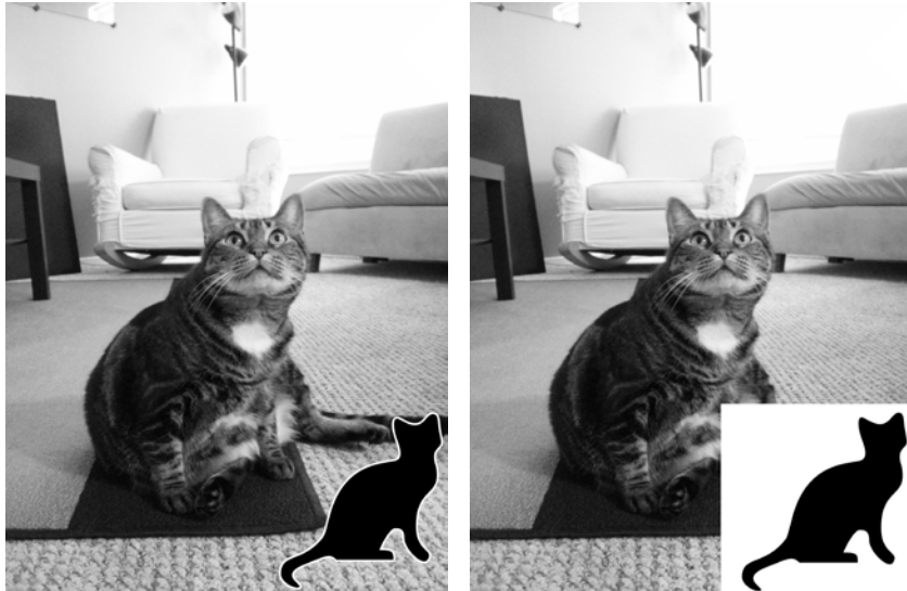
Figure 19-13: The image zophie.png resized and the logo added (left). If you forget the third argument, the transparent pixels in the logo will be copied as solid white pixels (right).
