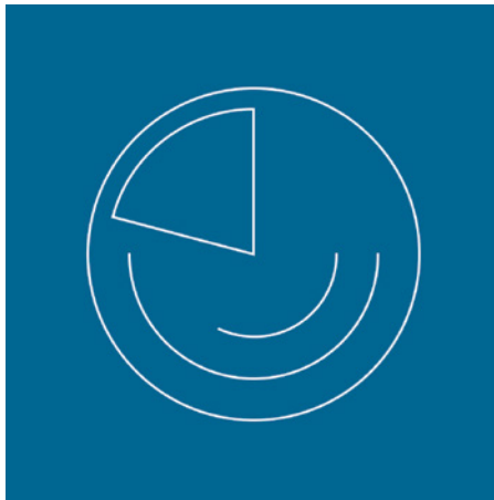
Figure 1-26: Here are four arcs, and one of them is a complete circle. The slice-like arc (upper left) uses the PIE argument.
