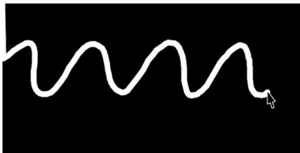
Figure 11-3: Drawing a continuous line by using a line() function for each frame
