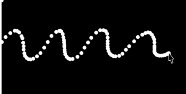
Figure 11-2: The faster you move your mouse, the larger the gaps in the line.
