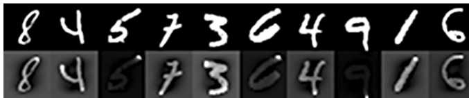
Figure 7-1: Original MNIST digits (top) and normalized versions used by the models (bottom)
