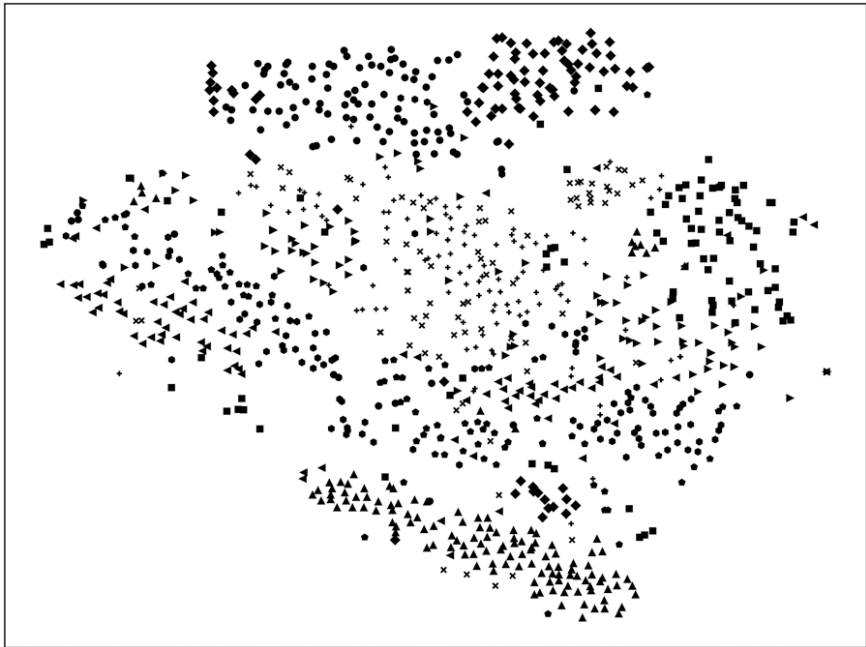
Figure 14-4: t-SNE plot showing the separation by class for the embedded MNIST digit vectors
