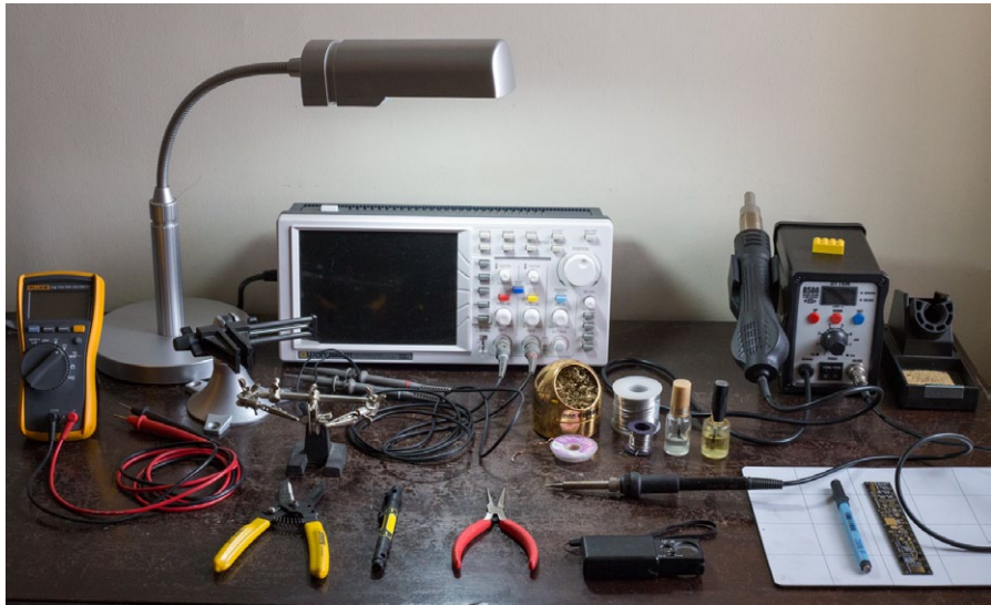
Figure B-2: A typical electronics workbench, with a multimeter, a task lamp, clamps, a wire stripper, a screwdriver, needle-nose pliers, a loupe, solder, flux, an oscilloscope, and a soldering station.
